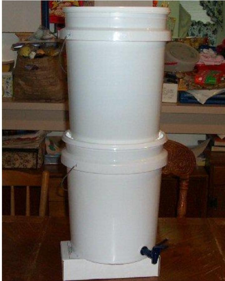
To use the filter, fill the upper bucket with water and wait. If you are starting with dry elements, it will take quite a while before the water starts dripping into the lower bucket. It takes up to several hours for the clean water to drain into the lower bucket. This process can be sped up considerably by frequently topping off the water in the upper bucket. This maintains maximum pressure on the elements.
