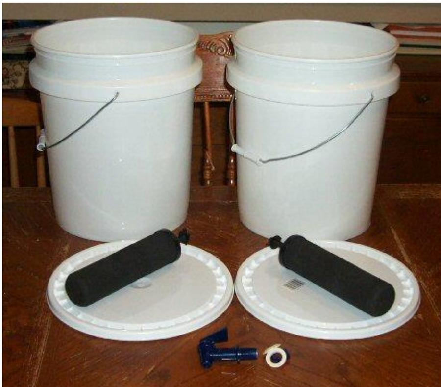
Drill two 1/2" holes in the bottom of the upper bucket and two matching holes in the lid of the lower bucket.
