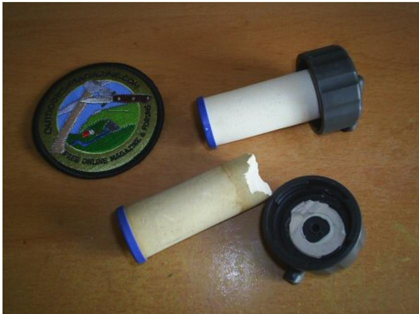
**A ceramic filter failure** The upper filter element is new; the filter element at the bottom is used and has obviously failed. The cause was either overpressure or a crack cause by an impact.
