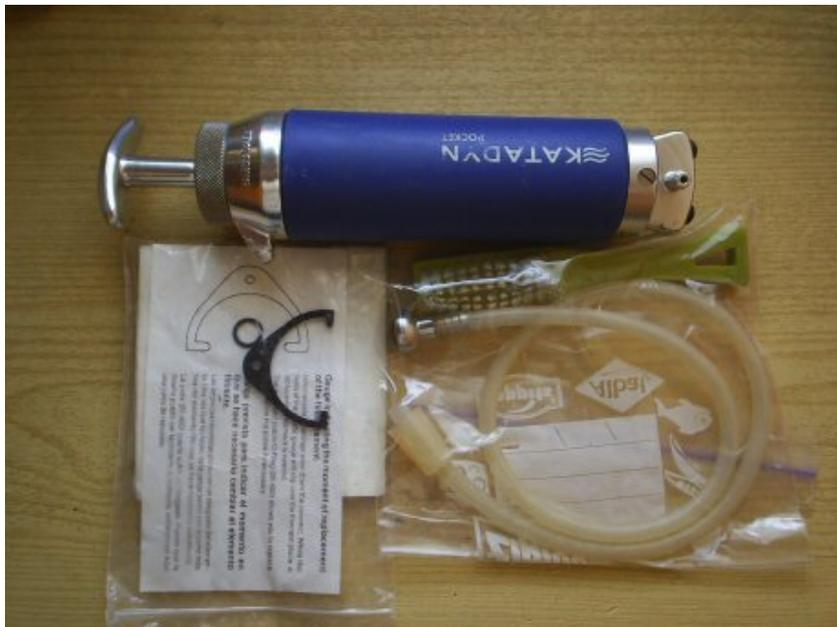
**Proper discipline prevents (cross) contamination of the hoses.** Packing the hoses separately in waterproof Ziploc bags is a one way to achieve this, clearly mark the dirty and clean bag!
