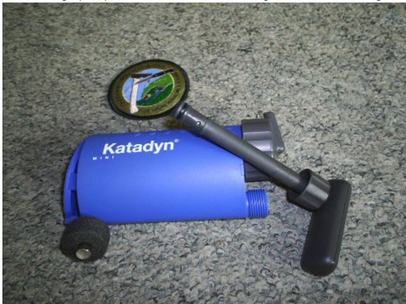
**A single action pump** Note the long and thin design of the pump rod; this makes it easier to pump than a "fat" pump rod.
