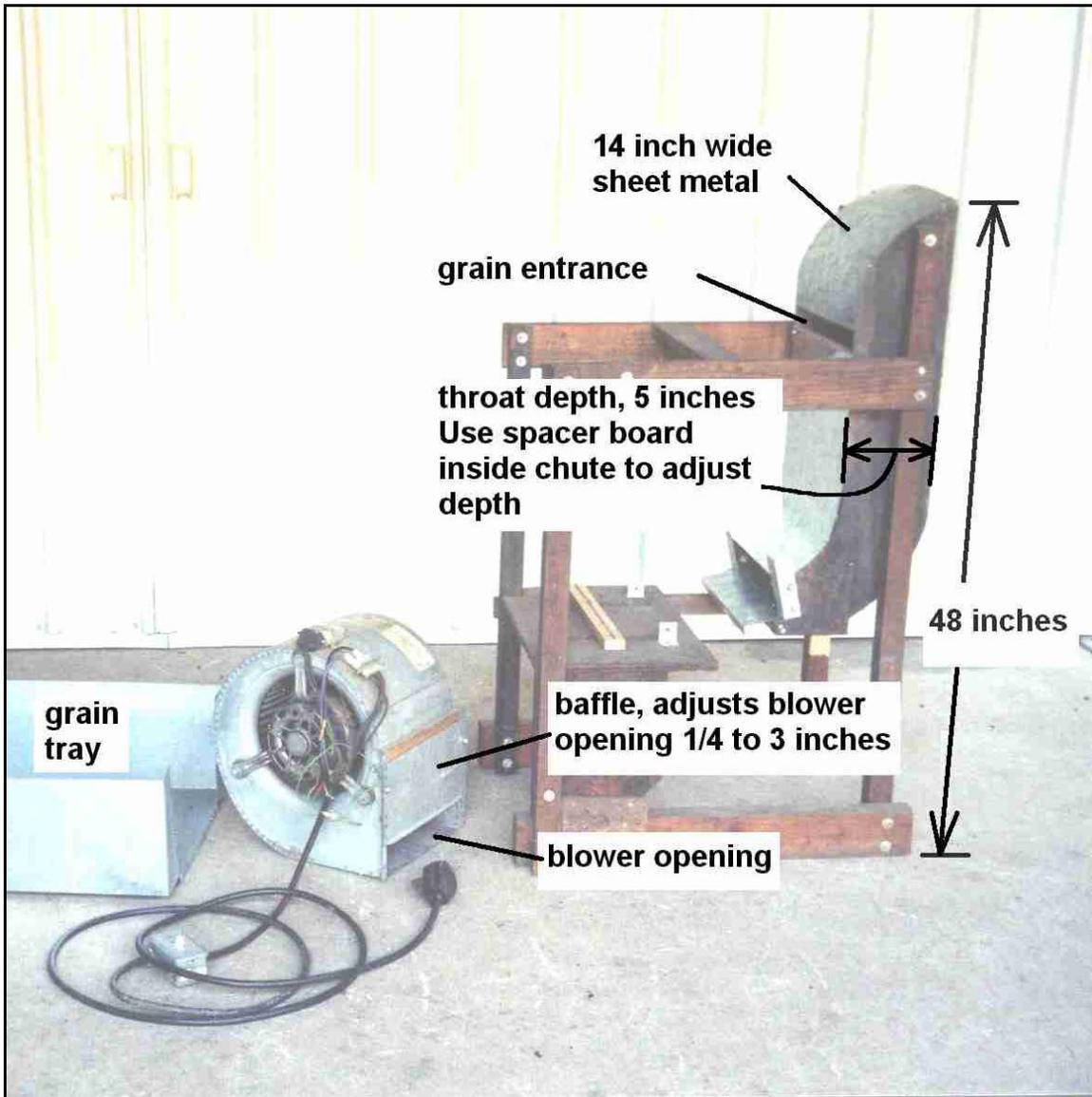
**Fig. 2 Winnower, disassembled**
