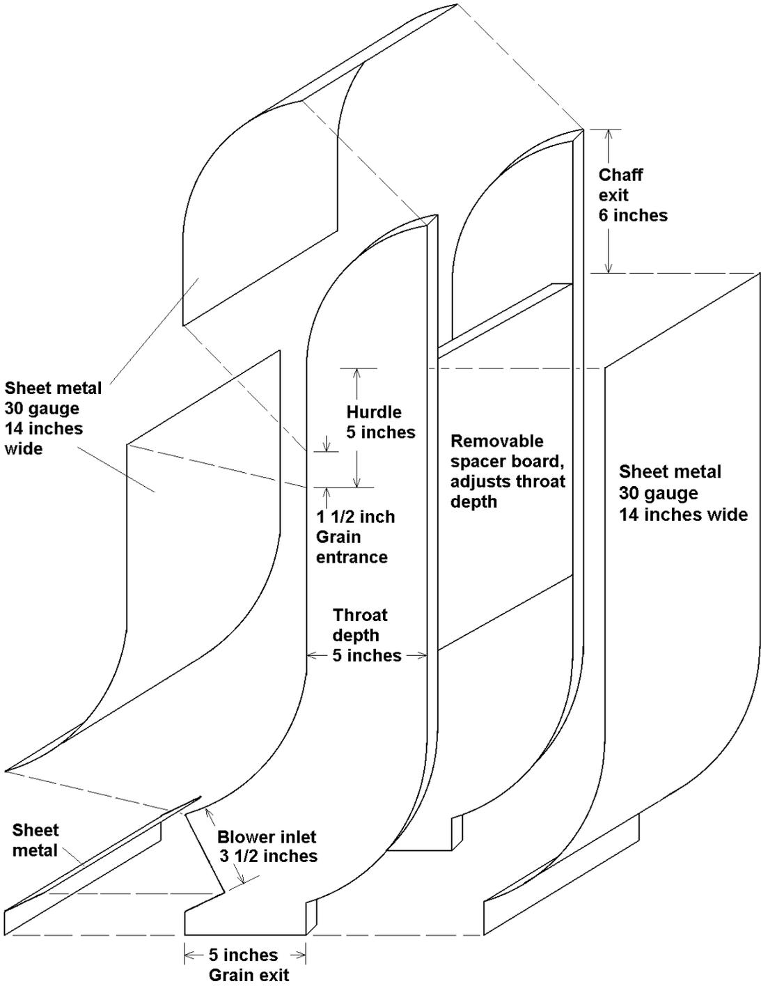
Figure 3. Exploded view of winnower chute
